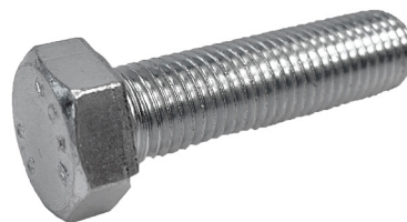
Parafuso cabeça hexagonal de aço carbono zincado com rosca total EN ISO 4017 (DIN 933) - Classe 8.8 - Carbon steel hexagonal head bolt with total thread and zinc coated EN ISO 4017 (DIN 933) - Class 8.8
