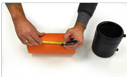
4. Medir a zona a raspar. Measure the scraping zone.
