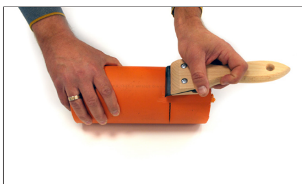
5. Raspar a zona de soldadura do tubo. Scrap the welding zone of the pipe.
